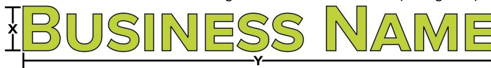
Figure 9 Wall Sign Area Calculation
