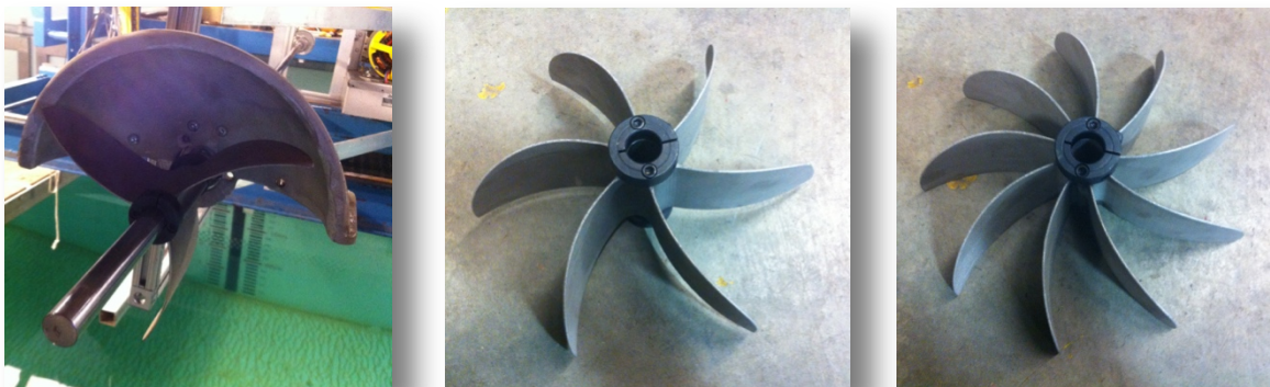
Figure 1 Model Turbines 3 blades with cowling, 6 blades and 9 blades
