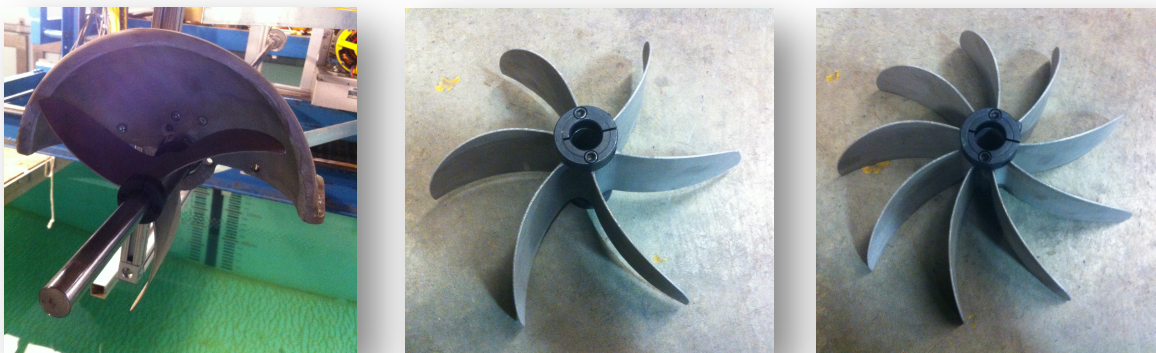
Figure 2 Model Turbines 3 blades with cowling, 6 blades and 9 blades
