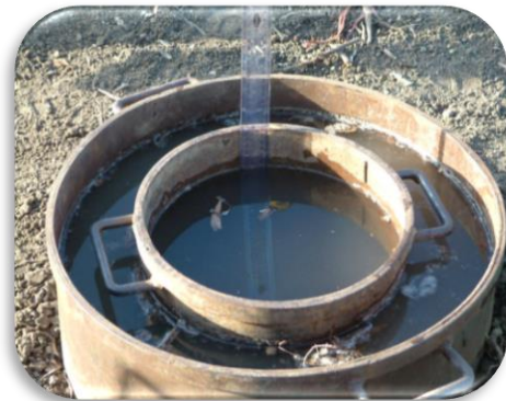
Figure 7-9: Double Ring Infiltrometer (Wikipedia, 2018)
